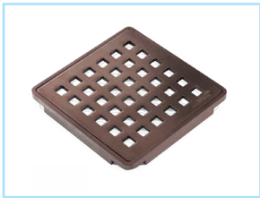
wedi Fundo® Drain Cover ORB Drain type: point Metal type: stainless steel 304 Coating: oil rubbed bronze Finish type: lightly brushed/buffed Size: 3 ¾ x 3 ¾ x ¼ in.
