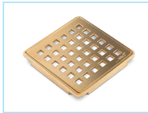
wedi Fundo® Drain Cover G Drain type: point Metal type: stainless steel 304 Coating: gold Finish type: lightly brushed/buffed Size: 3 ¾ x 3 ¾ x ¼ in.
