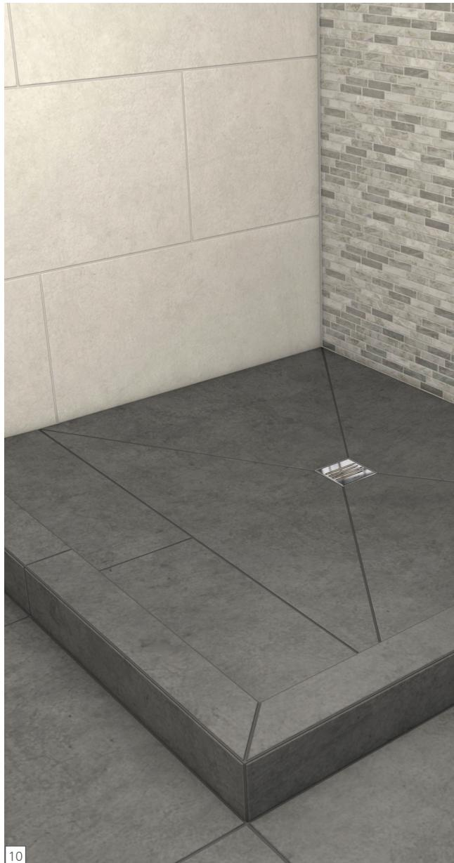
**EN** The shower unit is ready for tiling. Please consider and plan for the tile cut and grout line design. The shower base features slope fields that direct water to the drain from all sides, while the extension surface provides one sloped direction. For tile size recommendations and other post installation considerations please review the applicable Primo, Ligno, or Riolito Fundo Installation Manual, which applies to the extended shower floor area as well.
