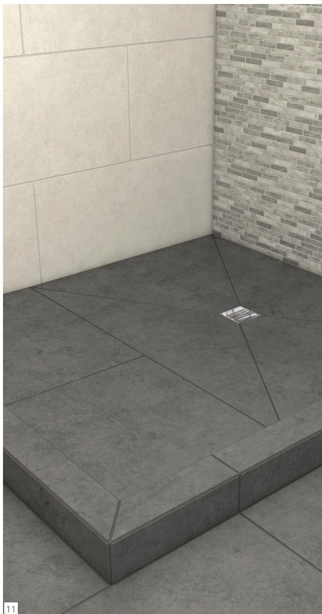
**EN** The shower unit is ready for tiling. Please consider and plan for the tile cut and grout line design. The shower base features slope fields that direct water to the drain from all sides, while the extension surface provides one sloped direction. For tile size recommendations and other post-installation considerations please review the applicable Primo, Ligno, or Rioli Fundo Installation Manual, which applies to the extended shower floor area as well.
