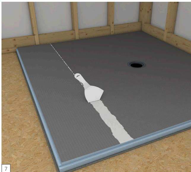
**EN** Finally, a continuous  $\frac{1}{2}$ " bead of wedi joint sealant is applied over all surface connection joints and spread over the joints using a putty knife.
