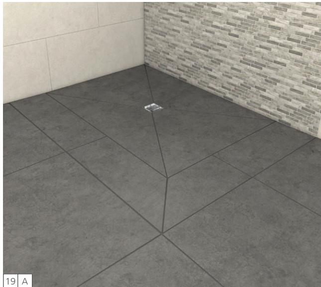
**EN** The shower unit is ready for tiling. Please consider and plan for the tile cut and grout line design. The shower base features slope fields that direct water to the drain from all sides, while the extension surface provides one sloped direction. For tile size recommendations and other post-installation considerations please review the applicable Primo, Ligno, or Riolito Fundo Installation Manual, which applies to the extended shower floor area as well.
