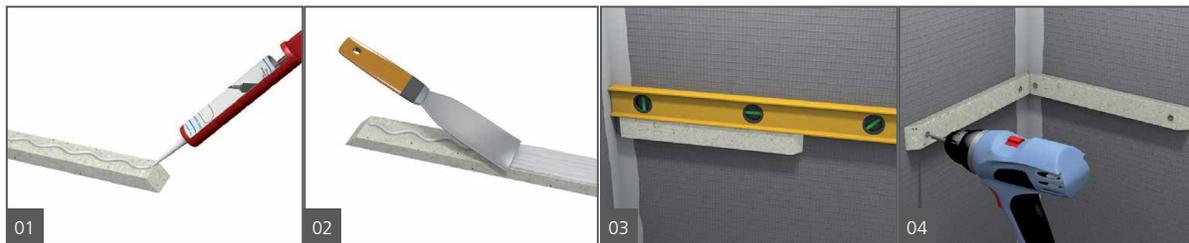
1. Apply wedi Joint Sealant to the side of the mounting bracket that will be attached to the wedi Building Panel wall.
