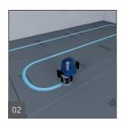
Cut grooves using a router. Cutting width should be the same as the pipe width; cutting depth should be at least 1/8" (3.2 mm) deeper. Make sure at minimum a remaining wedi Building Panel foam thickness of 1/4" (6.4 mm) remains intact below the pipe.
