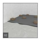
Stagger all joints when laying wedi Building Panels on the floor. Apply some weight on the boards during initial thinset setting time and especially over board transitions.
