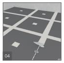
Tape all joints with wedi fiberglass mesh tape in dry areas or wedi Joint Sealant in wet areas. Fastener locations should be waterproofed too using wedi Joint Sealant. Begin tiling once tile adhesive has cured below wedi Building Panel.
