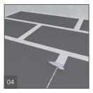
Tape all joints with wedi fiberglass mesh tape in dry areas or wedi Joint Sealant in wet areas. Begin tiling once thinset has cured below wedi Building Panel.
