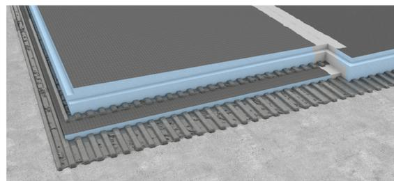
wedi shower bases thicker than 1 1/2 inch where an extension is connected require a wedi building panel be placed and thin-set mortar adhered under the extension panel to adjust for a proper connection fit.
