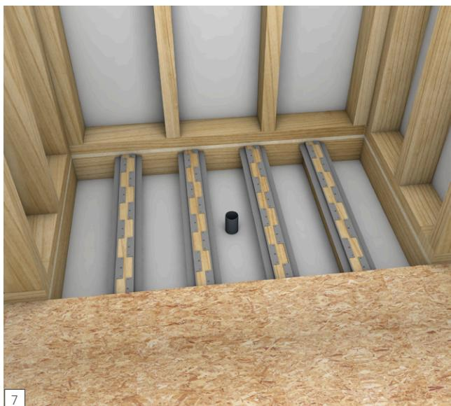
[EN] All floor joists have been equipped with a joist bracket on both sides.
