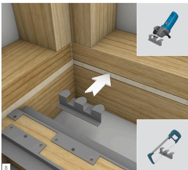
[EN] Place C brackets at the wall sides. The C brackets are installed at both ends of the recess area first and then along the wall / side every 12" (304.8 mm) (center of C bracket to center of C bracket).
