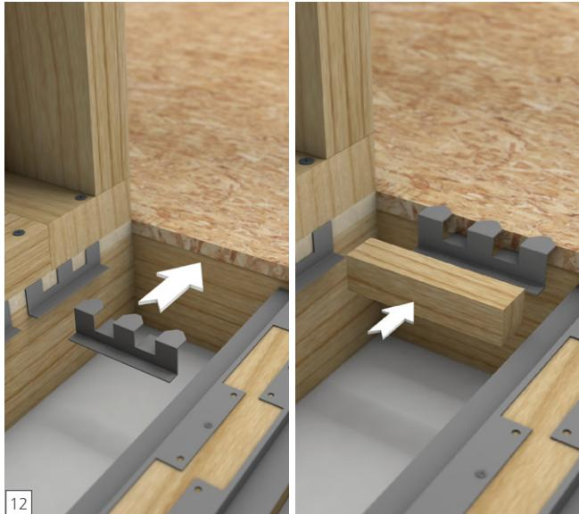
**EN** Dry fit C brackets to the edge of the wood floor to ensure C Brackets can be installed for full support along the edge of the floor plate. Use a wood block or hard rubber mallet to push the brackets in position.
