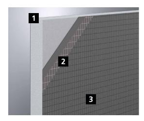
The wedi® BC Tile Backer's core is reinforced with fiberglass mesh embedded in a modified cement coating giving it extremely high tile backer bending strength and rigidity, as well a very high bond strength with common tile adhesives. What's more, the product's performance is moldproof, insulating, light and easy to cut and customize with a utility knife.
