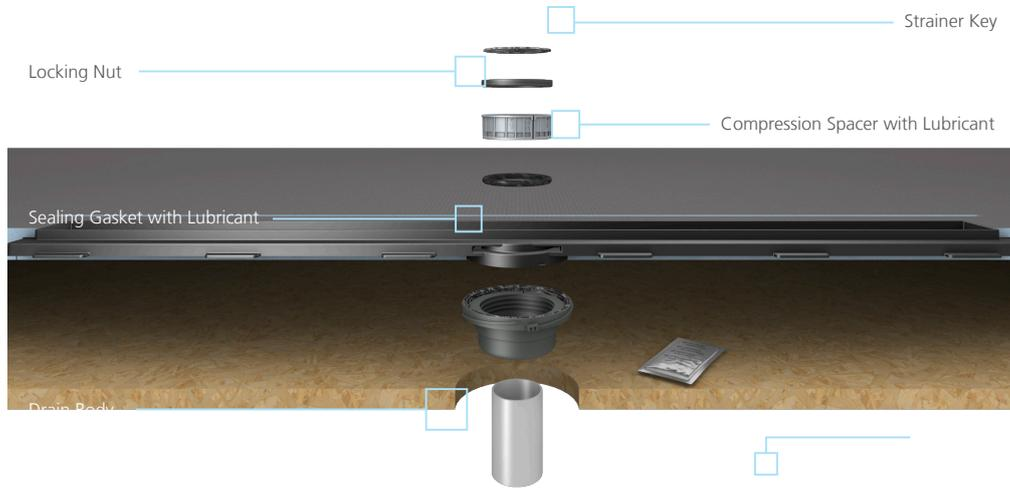
Use with nominal schedule 40 2 in. PVC, ABS or Cast iron waste pipe. Use special wedi parts for installation to copper pipe.
