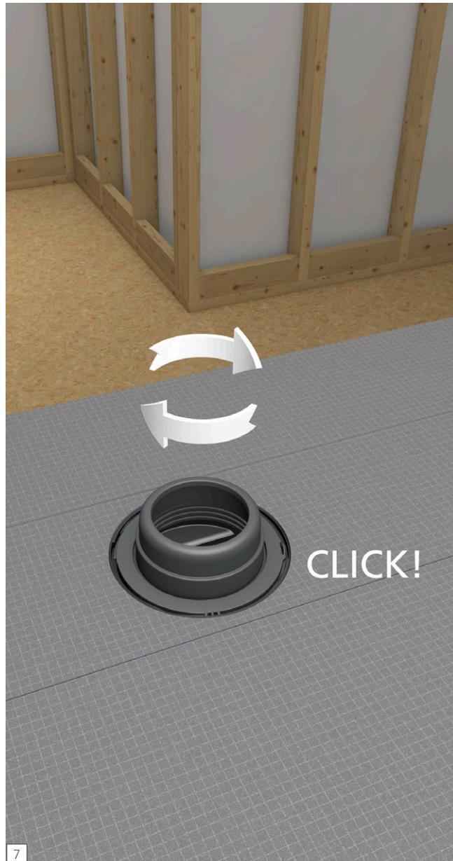
**EN** Insert the Drain Body snugly into the receiving mechanism of the Drain Unit on the underside of the Fundo base.
