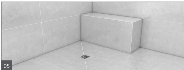
5. Start tiling immediately once sealant and thin set tile adhesive is dry to the touch.
