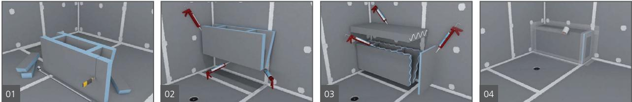
1. Cut the bench support and seat to length using a knife, handsaw, or circular saw.
